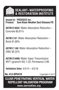
NOTE: The SWR Institute Validation Program uses standardized testing for validation purposes, including testing on CMU. PROSOCO does not recommend the use of Siloxane PD on CMU. Please reference the Substrate Chart on page 2.
